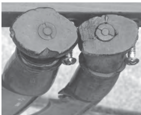
Picture 3: The two butt caps of the Mk.1s depicted in picture 1. Note the slotted round nut mounted flush, or semi-flush, to the butt of the Mk.1s. As far as I know, no other kukri uses this type of blade to handle attachment.
