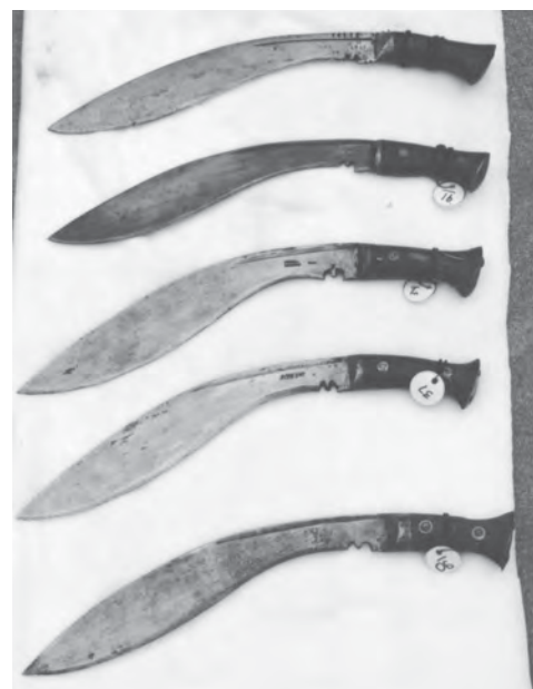
Picture 5: Mark 2 kukris that are all different contractors. They range in date of manufacture from 1919 to 1944. They are all similar in appearance, with the exception of the second from the top; and this is because of extensive sharpening. The two top earlier Mk. 2s have handle rings which were dropped after 1941 for the most part.
