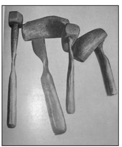
Tools? How about these hammers that were used in the 19th century? The ash wood handles show wear, in some specimens, of sixty years' continual use. Notice that a hammer used by a left-handed forger was so grooved from finger wear that it could not have been used by a right-handed worker. (specimens from the collections of the Sheffield Trades Historical Society and Mr. J.B. Himsworth)
