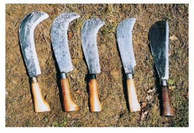
photo of a range of billhooks with a progression of curves and nose length. They are all of the simplest and commonest type, being single edged hooks, with tanged handles and a double sharpening bevel. All these billhooks would have been available in 9" or 10" blade length (some down to 8" and up to 12"). This selection includes both 9" and 10" hooks, only because they are what I have.
