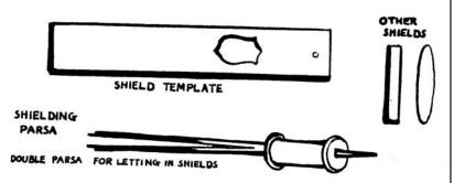
Two legged parser or shielding parser. A parser (q.v.) with a curious bit, consisting of two cutting legs sprung from a common joint, and mounted in the parser bobbin. These two legs open and close as the drill revolves, following the outline cut in a template, or shieldplate. Thus the cutler can cut a hole of any shape, square, diamond, etc., with a rotary drill, a feat engineers often say is impossible until they have seen it done.
