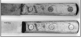
Verdigris has formed around the brass rivets of this old Barr Bros knife. When the verdigris was removed, the knife was like new again.
