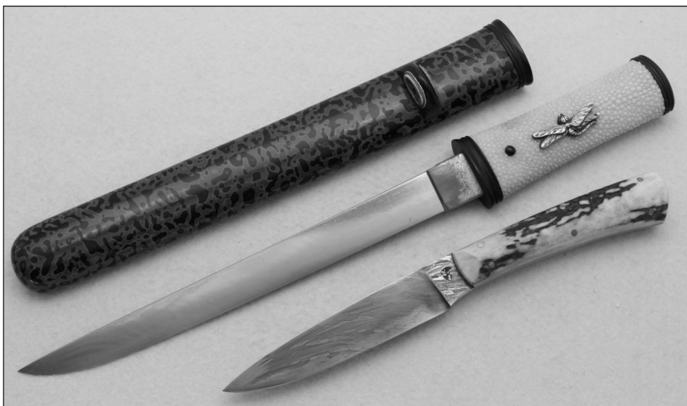
These two pieces were made from cable Damascus. The tanto was made in 2007 and the sheath knife in 1994.
