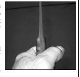
the rusty blade and the now nice handle was just too great. I thought I could just give the blade a few quick passes on the belt sander, and that should do it. Well, I found out that the pits were a little deeper than I realized. The quick touchup effort turned into a lengthy grinding job. Being a 12 inch blade, there was a lot of surface area to address; and the rust pits were evenly distributed on all surfaces. There was no turning back at this point. I had to finish the job.
