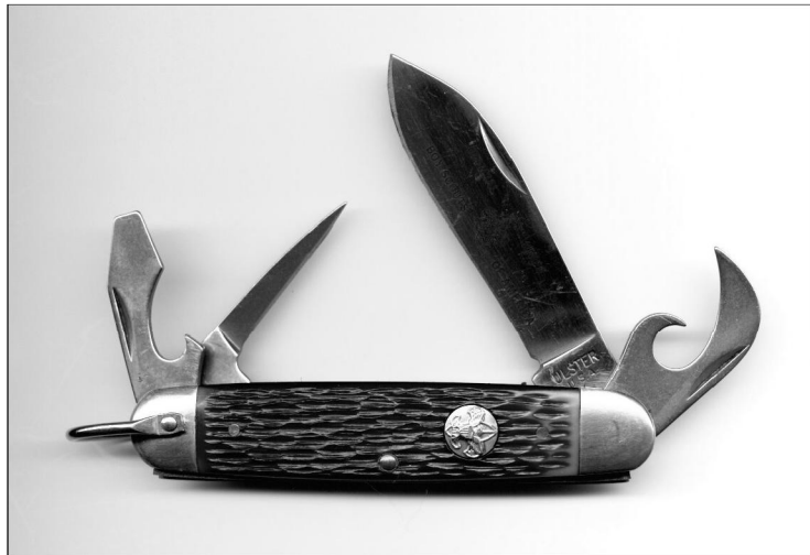
This is a close up view of the Swinden Key construction. Notice the large head on the rivet that is holding the blade/liner assembly together.
