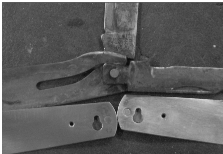
This view shows the rivet heads a bit better. They fit into the keyway in the outer liner/bolster assembly.
