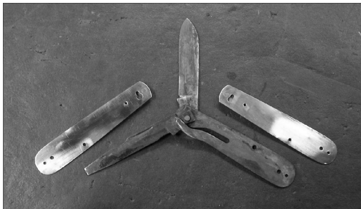
This is a close up view of the Swinden Key construction. Notice the large head on the rivet that is holding the blade/liner assembly together.
