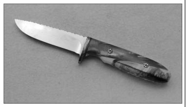
pattern. The steel is 1095 and is .125" thick. Larry has been the driving force for the knife grinding competition for many years, and this is the first time he has used one of his very own design patterns. Larry profiled 12 blanks for the competition.
