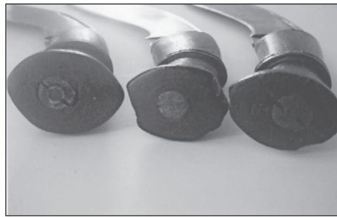
Picture 3 -Three butt caps of the Mark 1 kukris shown in Picture 1. Note the slotted, round nuts mounted flush or semi-flush to the butt of the Mark 1s. Picture courtesy of Simon Hengly, Tora Blades.
