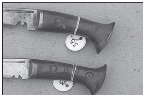
Diagram 2 -A half-tang kukri, the blade is secured in the handle by a homemade epoxy. Some of the ingredients are natural saps and pitches found in Nepal's forests and jungles.
