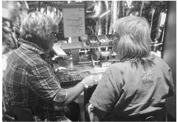
Karina (left) supervises as Sheree assembles her Victorinox Spartan. Small parts are in trays at the front of the bench. The press is clearly visible in front of Sheree.
