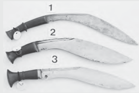
#7) (1) and (3) hand engraved fuller (1) very early (1820s) (3) much later possibly 1950s (2) Nepalese having hand forged fullers
