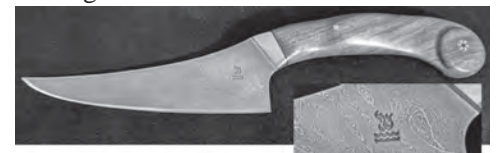
I've made a number of kitchen knives on variations of this design. This kitchen utility has a blade of homemade random Damascus in 1095/15N20. Vulcanized fiber spacers and brass bolster. Bubinga handle with Sally Martin mosaic pin.
