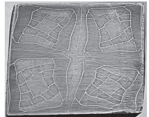
Image 3 A very early mosaic billet. The "bird" in the middle was created by trying to square up four stacked billets that weren't. No squaring dies were available.
