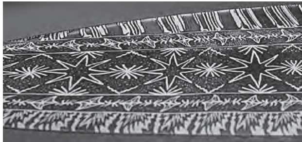
Image 5 A multi-bar blade with a central explosion pattern. Created by Swedish maker Connie Persson. Picture from Art And Design Of Modern Fixed Blade Knives by David Darrom, Pg 218.
