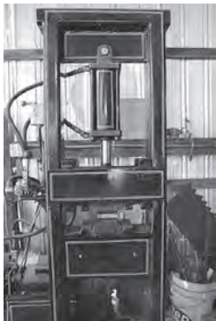
Knifemaker's hydraulic press
