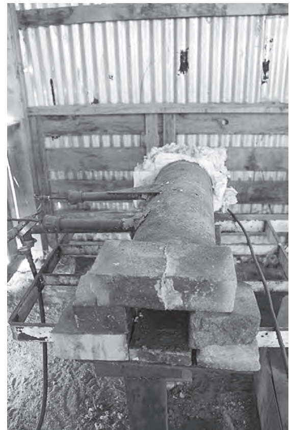
Two burner propane forge. The Kaowool at the rear is backed by fire brick, in case I want to open a back door
