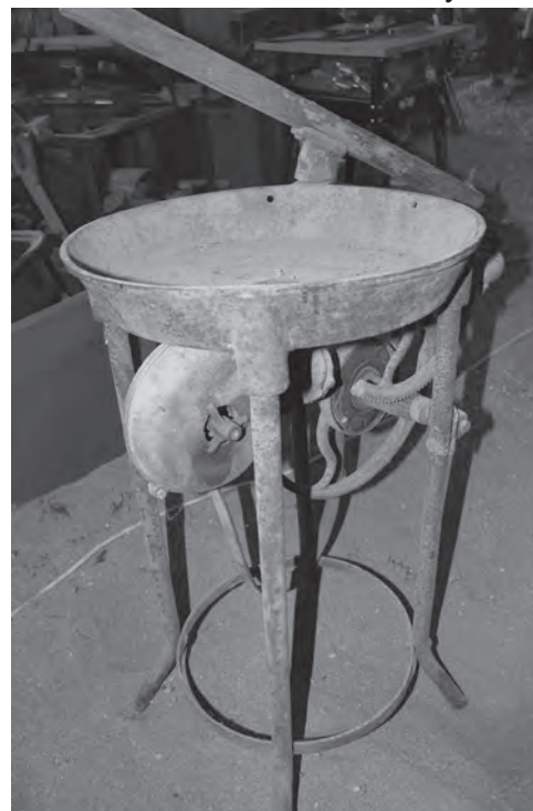
Pump handle forge. The pump handle drives the blower, rather than a hand crank. It uses a ratchet to turn continuously in one direction when pumped.
