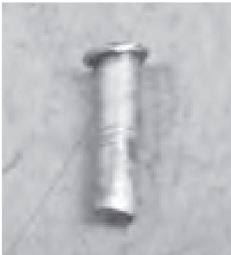
This a pin that has been peened wrong. It won't hold when the cap is removed.
