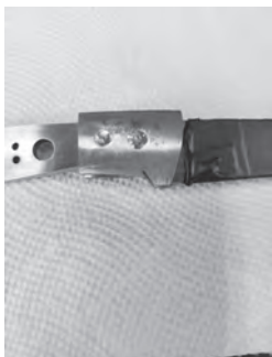
Copper pins after peening. For reference, those are 3/32 pins.
