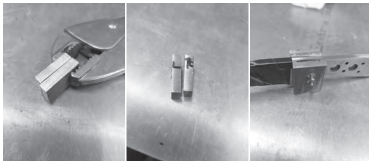
The second bolster ready to drill, faces indexed. I label sides to avoid beveling the sides wrong. Bolsters countersunk, beginning the peening process.
