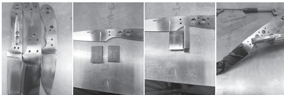
Pin patterns for bolsters. Nickel silver pieces for bolsters. Flattened and ends squared. Clamped and ready to drill.
