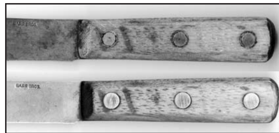
Verdigris has formed around the brass rivets of this old Barr Bros knife. When the verdigris was removed, the knife was like new again.
